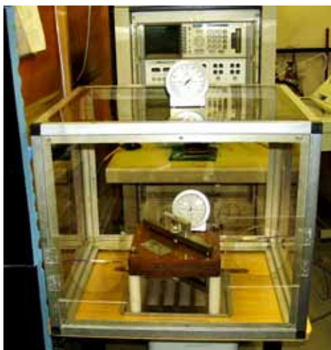
Fig. 9 Dry-air circulating system using moisture removal machine.
