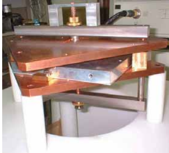
Photo. 3. Test cavity resonator operating at 1 GHz using aluminum side wall. (Courtesy of Keycom Co., Ltd.)
