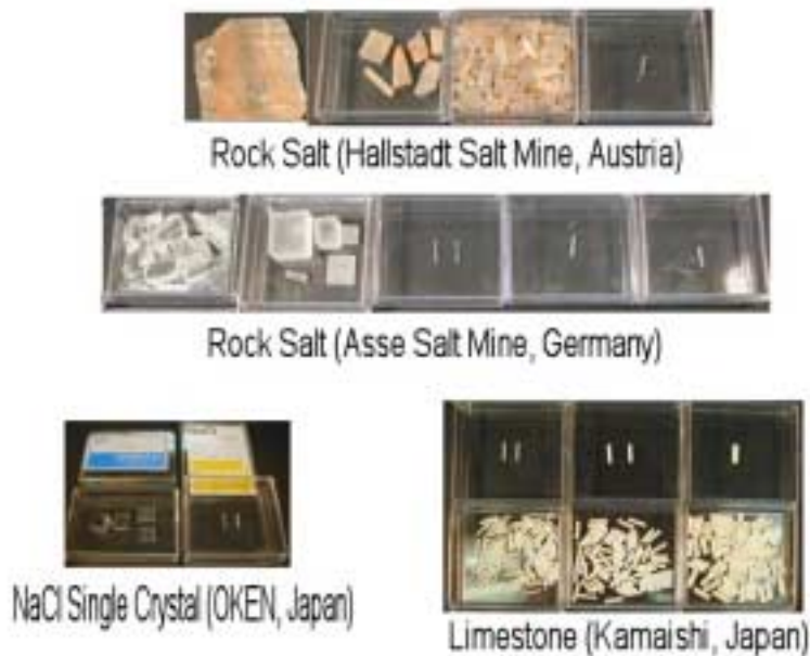
Fig. 8 Samples measured with the perturbative cavity resonator
