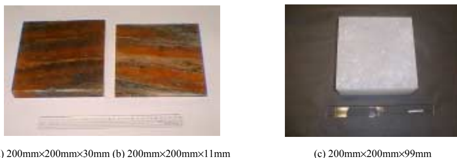
Fig. 2 Photos of rock salt samples from (a), (b) the Hallstadt salt mine, Austria, and (c) the Asse salt mine, Germany. The samples from the Hallstadt salt mine are brown in color and have a striped pattern to their coloration. The sample from the Asse salt mine is white and has no striped pattern. The rock salt appears to consist of small single crystals.
