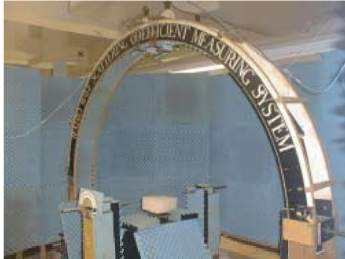
Fig. 4 Photograph of the measuring apparatus operating in the X-band with a sample from the Asse salt mine. The transmitting and receiving horn antennas are set on a 2.6 m diameter arch above the samples such that both the incident and reflection angles are 5^\circ .
